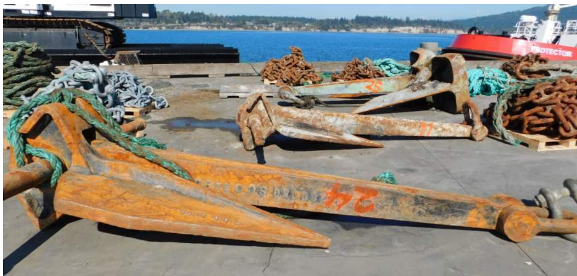
Figure 7.6 – Salvaged anchors showing different anchor types (Two Danforths in front, One Eells in back) (Source: Mott MacDonald)
