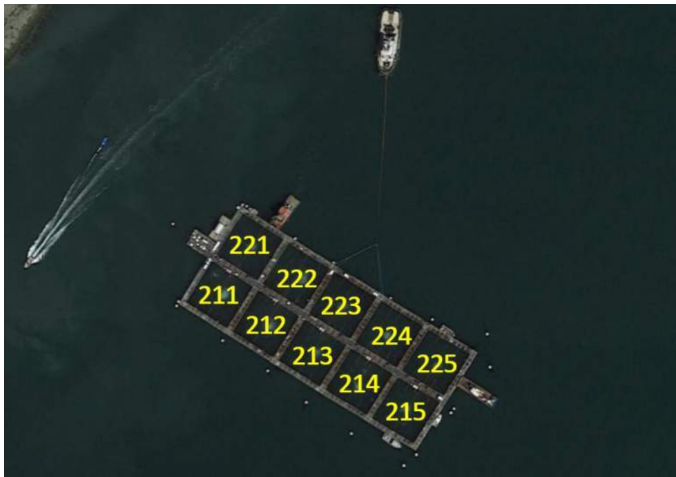
Figure 4.4 – Net Pen #2 showing the ten cages. (Source: Google Earth) Photo is from July 25, and shows the tug, towards the top of the picture, stabilizing the net pen facility. Also appearing in the picture are the Cooke work vessels outside cages 221 and 225.
