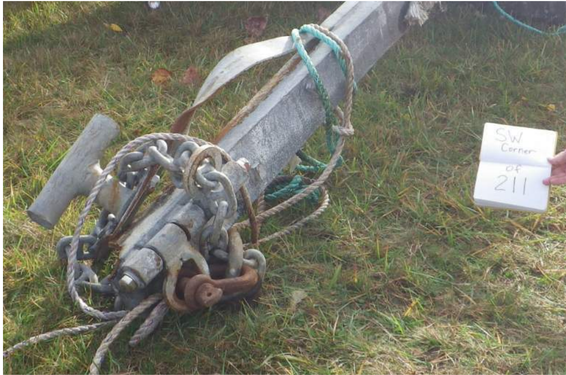
Figure 7.8 – Failed Outrigger Float section (Source: Mott MacDonald)
