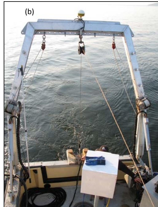
Figure 2-6. The R/V Brendan D II is equipped with a weighted towfish that contains an underwater video camera mounted in a ‘downward looking’ orientation, dual lasers for scaling reference, and underwater lights for night work (a). The towfish is deployed directly beneath the DGPS antenna attached to the A-frame cargo boom, ensuring accurate geographic location of the camera (b).
