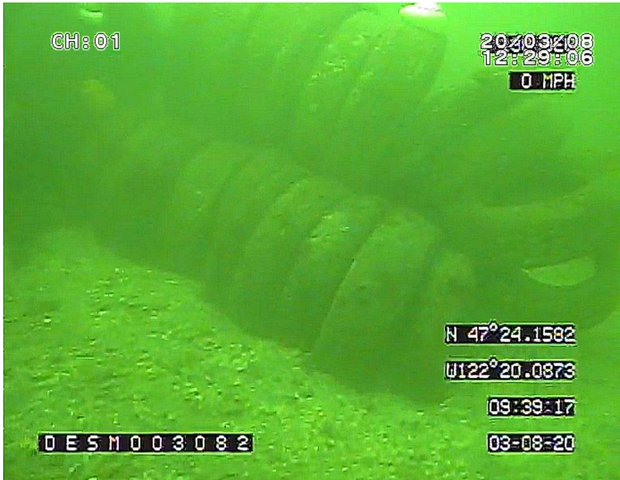
Figure 70. Side view of a pyramid – barrel stacked tire bundle (2 barrel stacked rows at base with one on top). Each row in the bundle appears to have 8 to 10 tires. We estimate the total tire count in this bundle to be 24 to 30 standard automobile tires.
