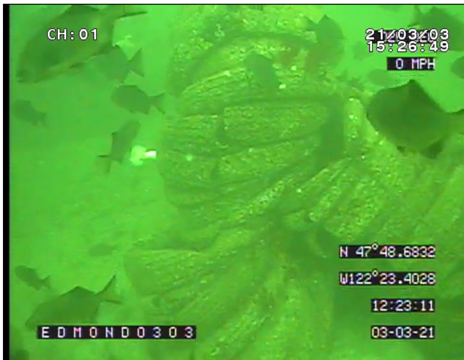
Figure 34. Organized barrel groupings of 6 to 7 tires per row for an overall tire count of 18 to 21 tires in frame.
