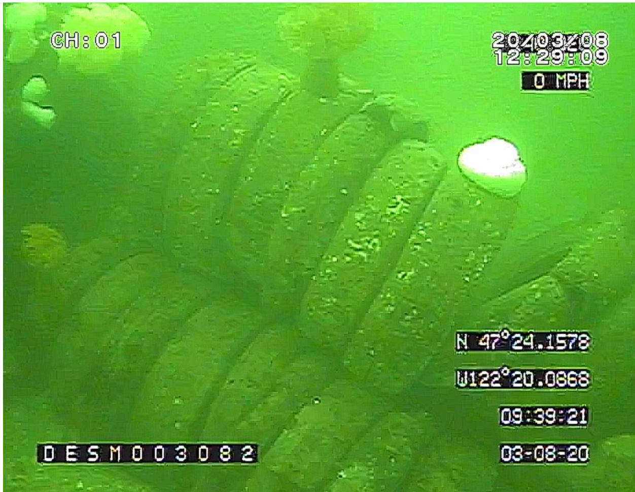
Figure 71. Top view of a barrel stacked bundle pyramid of tires. Pyramids of this nature are the prevailing tire feature at the Des Moines site. Tires at the lower level here appear to be buried 15-20%.
