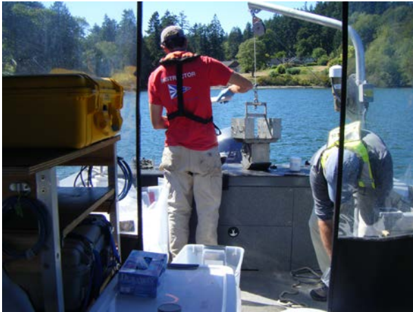
A downrigger was used to take sediment samples.
