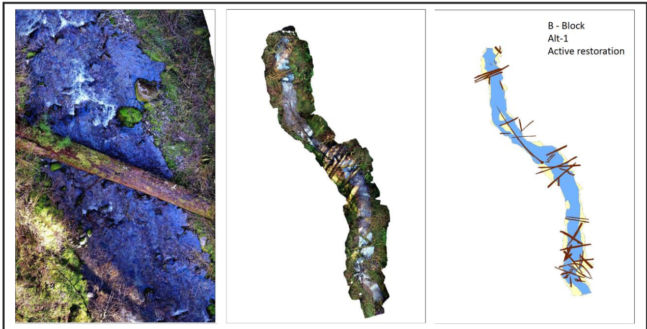
Figure 12. Drone photo image, photo mosaic, and resulting spatially explicit map of a studied T3 stream reach (left to right). (source: K. Martens)
