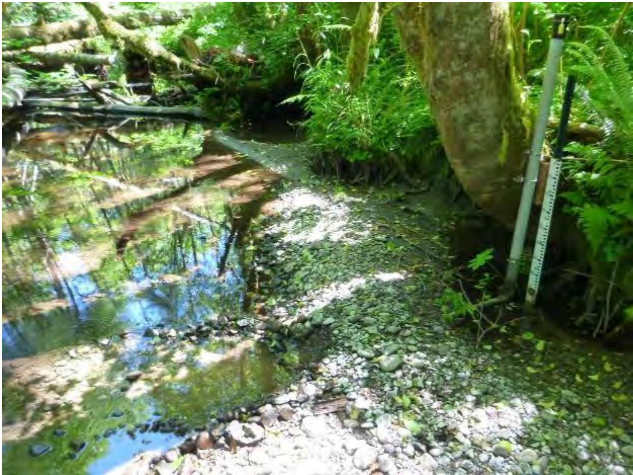
Stream gage station in basin 433 at low flow. Note the gravel bar formed around the gages after November 2014.
