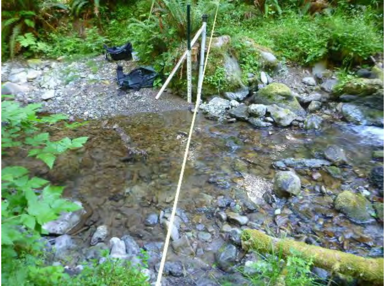
Stream gage station in basin 790 (measurement tape marks the location of the discharge measurements).
