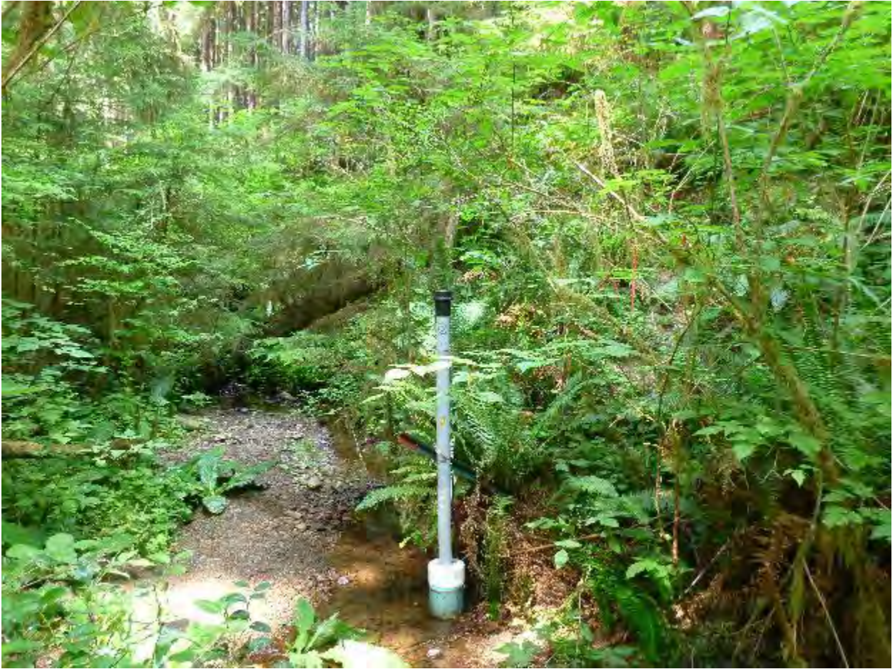
Stream gage station in basin 769 at low flow (the removable staff gage is not shown).
