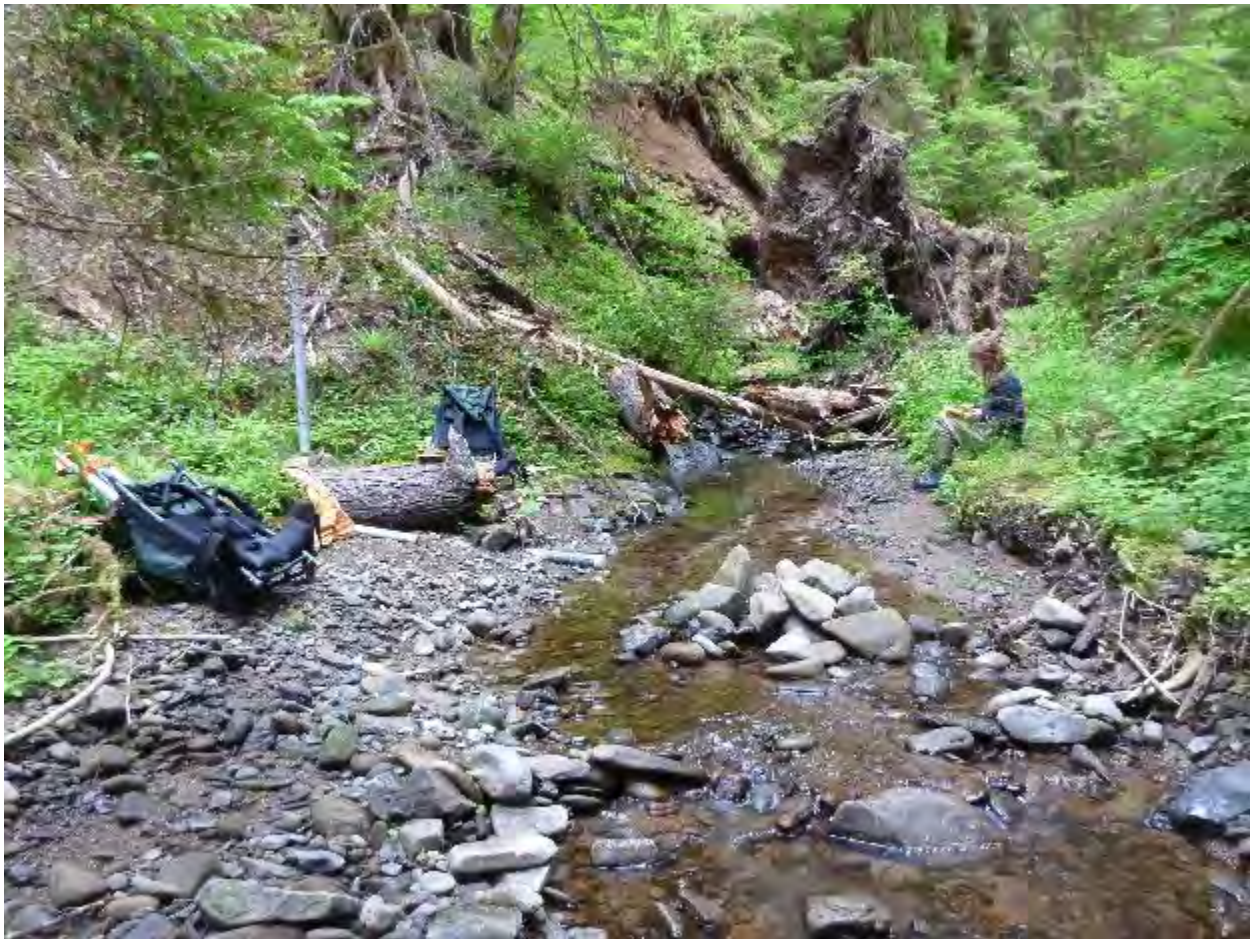
Stream gage station in basin 724 at low flow (the removable staff gage is not shown). Note the large tree which fell above the gage station in the winter of 2014/2015 and altered the channel flow.
