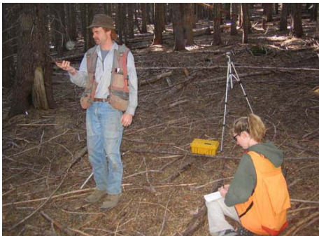
Comparing a densiometer and a fish-eye lens digital camera for measuring canopy closure.
