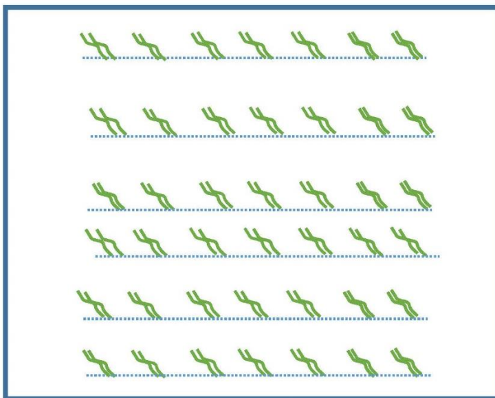
Figure 2. Example of planted 1 meter quad with 6 PU's (strips of burlap with eelgrass)
