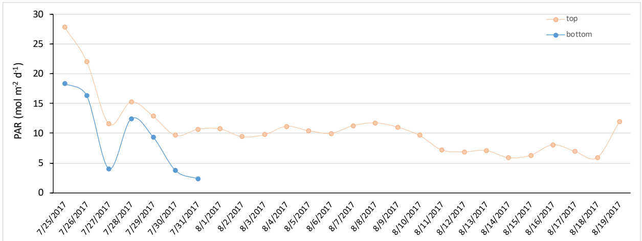
Figure 25. Photosynthetically Active Radiation (PAR) measured 15 cm (bottom) above the sediment surface between July 25 to August 19, 2017, at an eelgrass test-transplant plot at Joemma Beach State Park. The bottom sensor failed to record data consistently after July 31, 2017, therefore, these data are not presented.
