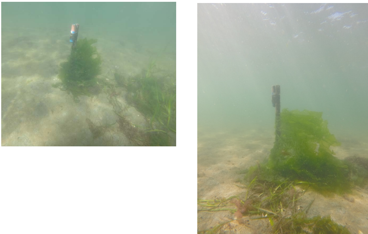
Photograph 8. Photographs of the PAR sensors that show the bottom sensor fouled by green algae (ulvoids). The low PAR values recorded when a sensor was fouled creates an unrealistically high attenuation value ( K_d > 5 ).
