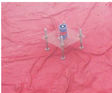
Figure 4. Submerged light (PAR) sensor supported by Plexiglas mount at bottom at AQUA tank.
