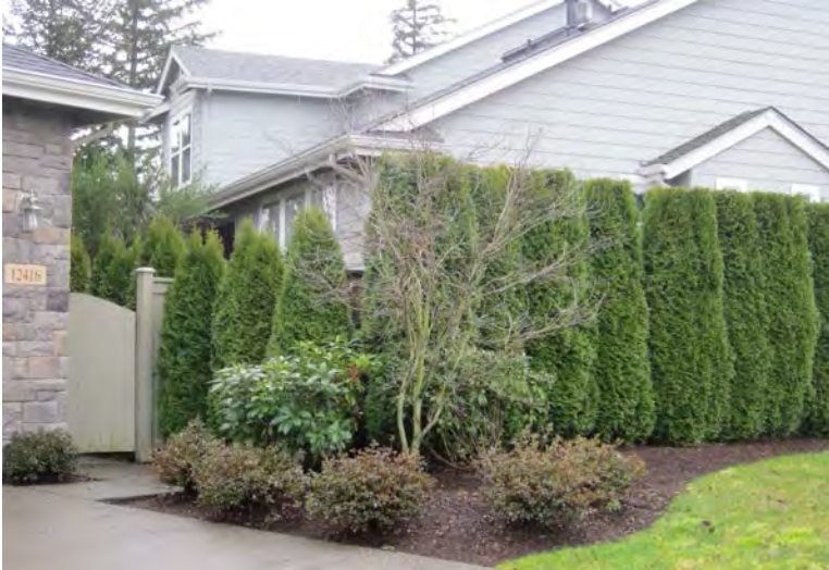
Figure 5-13: Flammable privacy plantings near home and connected to the wooden fence.
