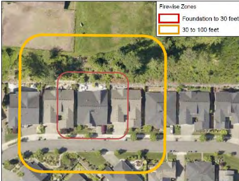
Figure 3-1: Example of Firewise Zones in Trilogy at Redmond Ridge. Neighboring properties can have interconnected zones.
