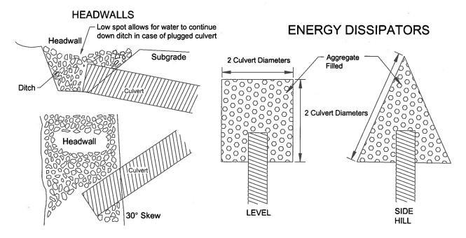
Headwalls to be constructed of material that will resist erosion.
