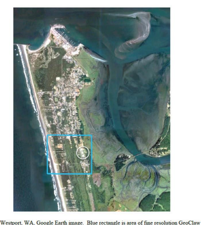
tsunami model grid; white circle encompasses Ocosta School campus. Study funded by Washington State Emergency Management Division The next step was to do high-resolution tsunami inundation modeling to define the required height of the structure and to estimate the loads the structure would be designed to resist.
