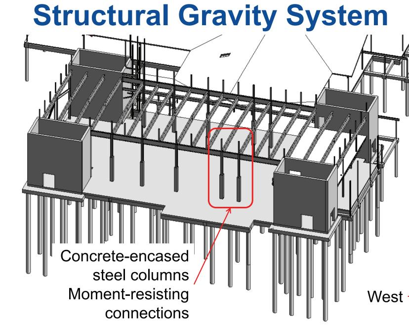
The details of the structural system are shown above. The gym will be pile-supported, with concrete shear walls and and columns with moment resisting connections. This design resists the maximum considered hydrostatic, hydrodynamic, and impact loads and to guard against progressive collapse.
