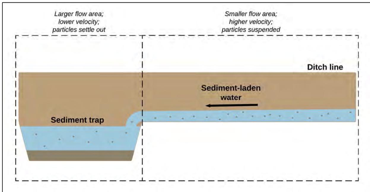
**Figure 1.** Ditch line with sediment trap schematic. In the ditch line, the flow area is small, which means the velocity of the sediment-laden water is high. Once this water hits the sediment trap, the velocity decreases because the flow area increases, thus allowing the sediment particles to settle out.
