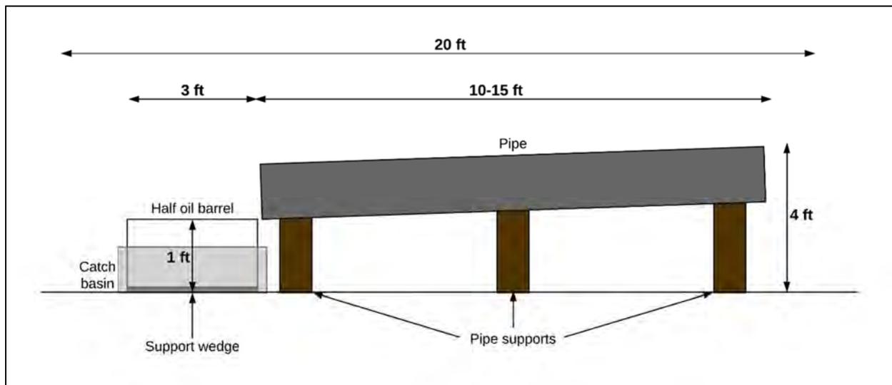
Figure 2. Experimental setup schematic.
