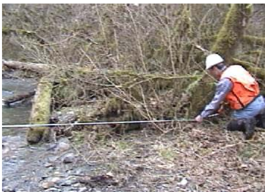
Forest Practices Compliance Monitoring Team member measuring the ‘bank full width’ of the stream
