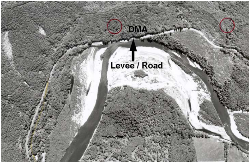
Figure 19. CMZ disconnected by a public right-of-way.
