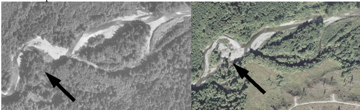
Figures 18a and 18b. Channel avulsion that occurred between two photo years.
