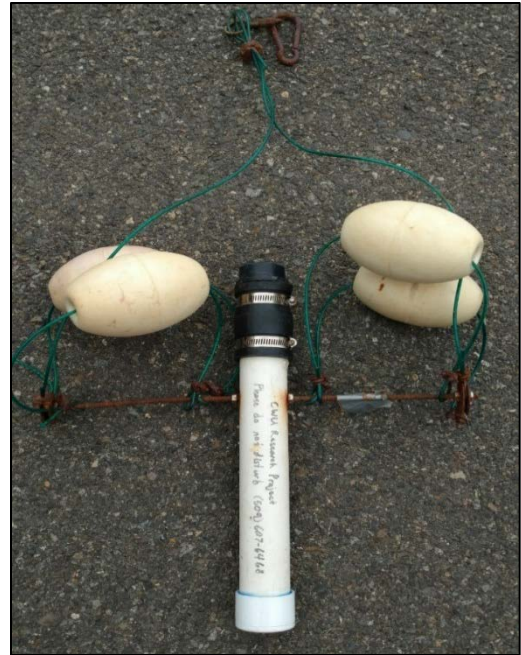
Figure 10. Floating PAR sensor rig for 1 cm from surface readings.
