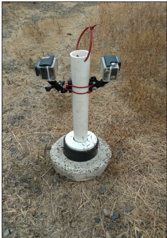
Figure 17. GoPro video set-up for fish use monitoring.
