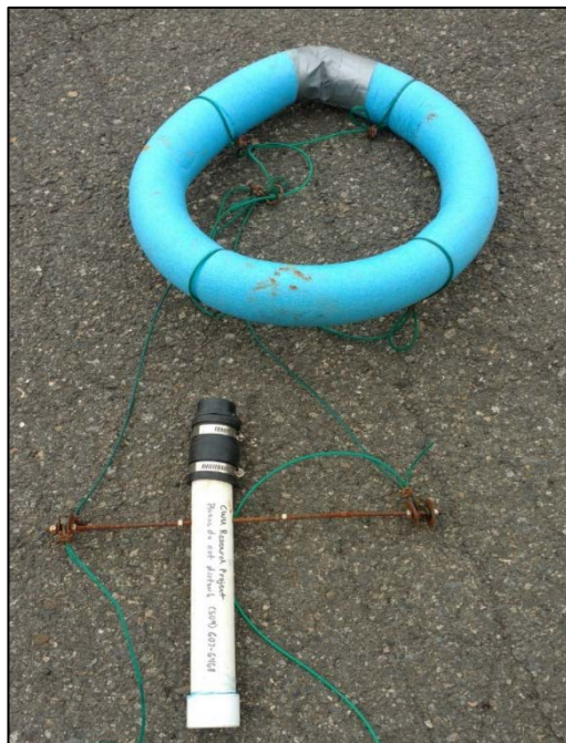
Figure 11. Floating PAR sensor rig for 1 m from surface readings.
