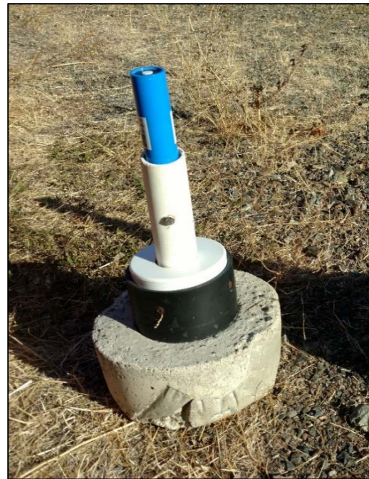
Figure 12. Benthic PAR sensor rig for seafloor readings.
